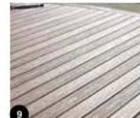
Composite wood decking, color & finish TBD (Stage)
